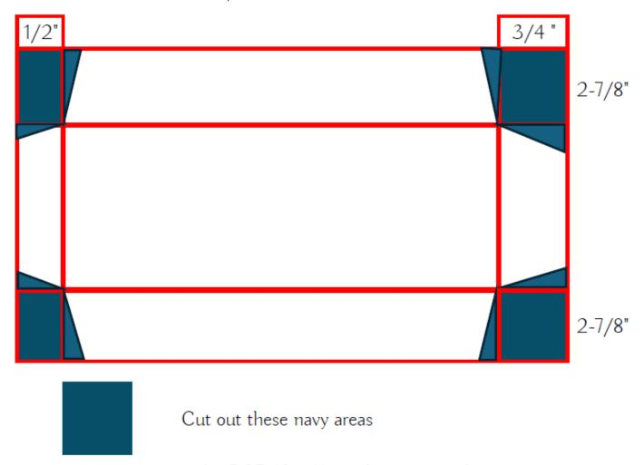
Directions for cutting away the DSP 10  $\times$  11 are the same as above using correct scoring measurements
